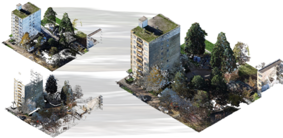
Fusing photogrammetric data with laser scanner data provides a detailed image of complex scenarios
